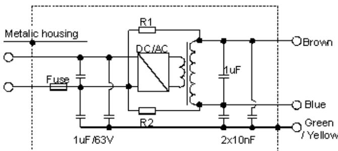
R1=R2= 2,7M ohm (not existing in SOLO 12V/200W, SOLO 24V/300W, SOLO 48V/300W)
