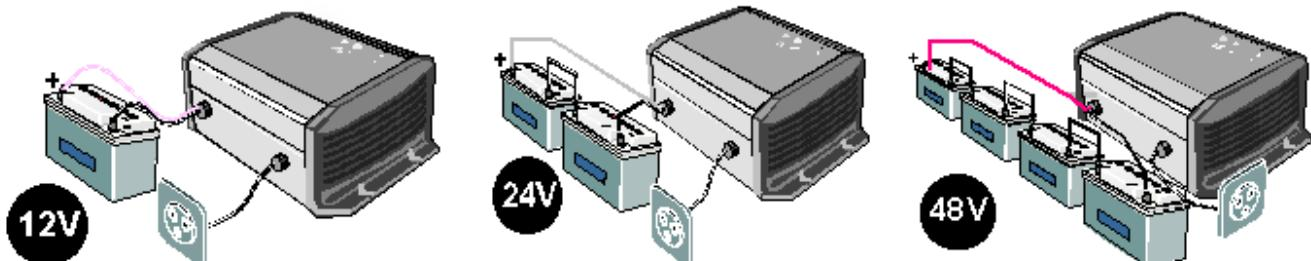
When connecting the battery, there's a spark (**Danger of explosion!**), because of the charging of the internal capacitor. Check that the cables are well adjusted. As long as it is possible, do not extend the cables supplied with the batteries. Extending them may increase the losses and cause malfunction of the inverter.
