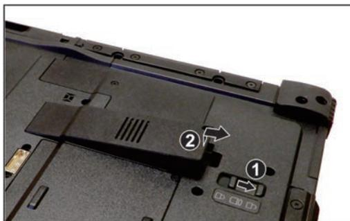
5. Insérez le nouveau module SSD en position. The security latch should be engaged in the locked position (🔒).
